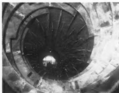
Interior of shell of "XH" Ruggles-Coles Dryer showing lifting flights and feed spirals.
